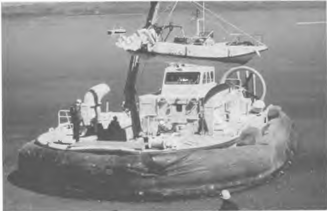
Figure 4. The hydraulic crane and well deck design of the Waban Aki enable the craft to support a broad range of response activities.
