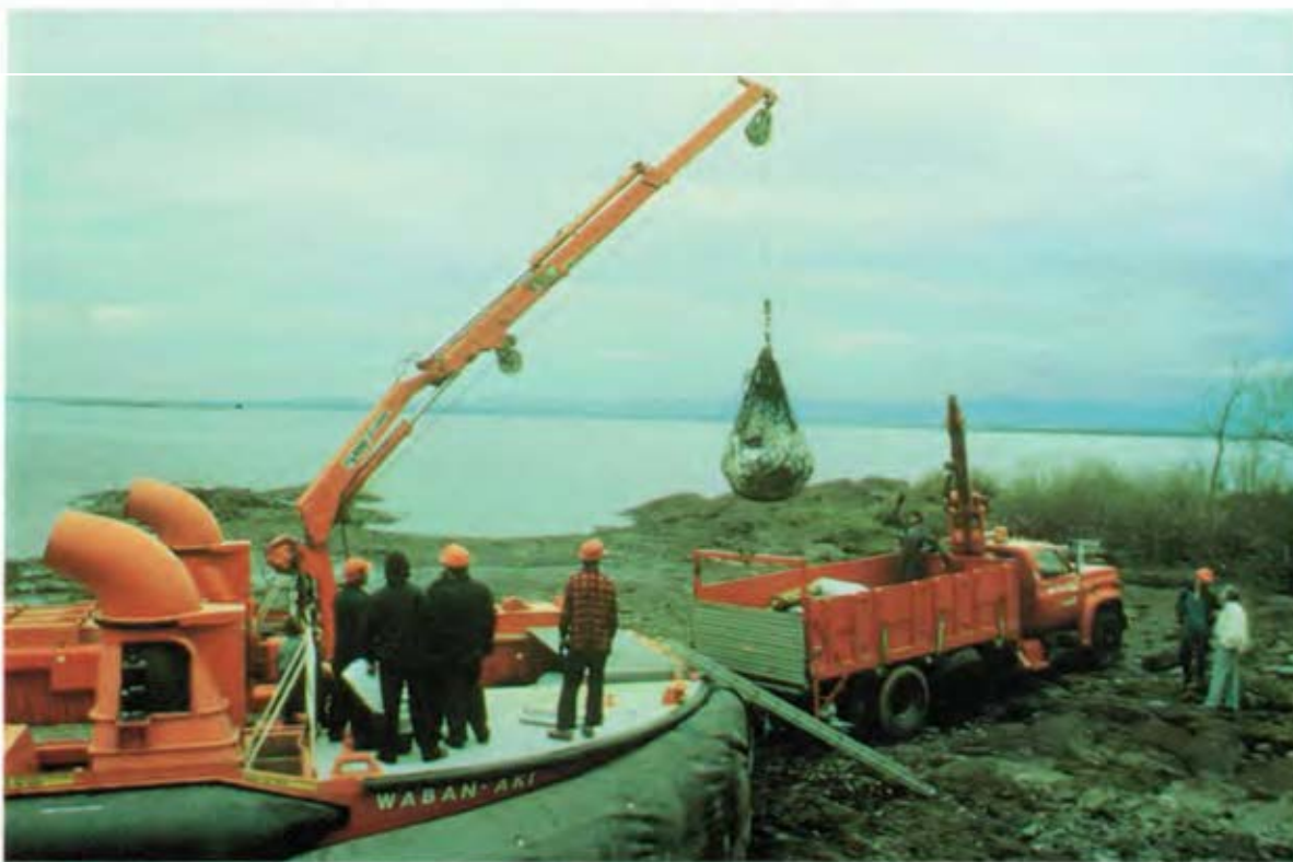
Fig. 1 The AP 1-88.250 uses its deck crane to handle cargo during the Rio Orinoco incident.
