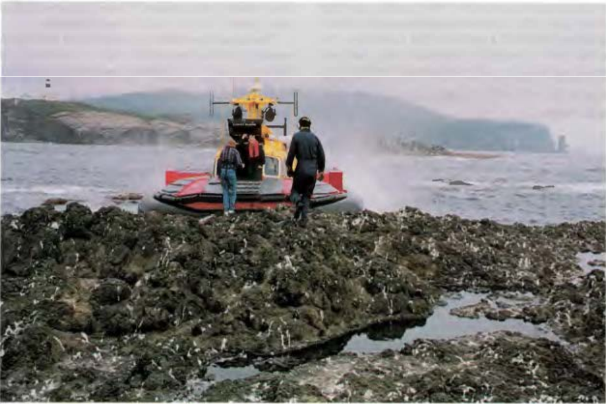
Fig. 3 Dynamically holding position to the swell, the SR.N-6 embarks a biological assessment team at a marine mammal rookery during the Tenyo Maru incident.
